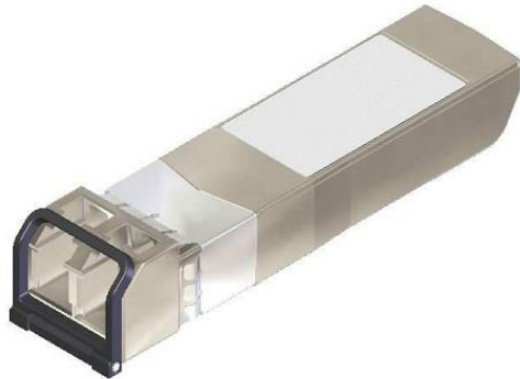
VCSEL based high speed (10 Gbps) SFP+ Module
