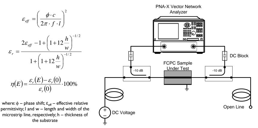
To eliminate the influence of the DC voltage source and open end of coaxial line on the opposite side additional time-domain data processing was used. It was possible thanks to signal delay caused by 3 m long coaxial cables and broad measurement frequency band.
