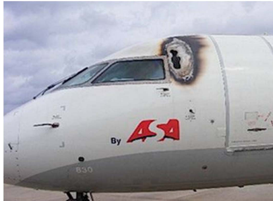
Lightning strike damage
